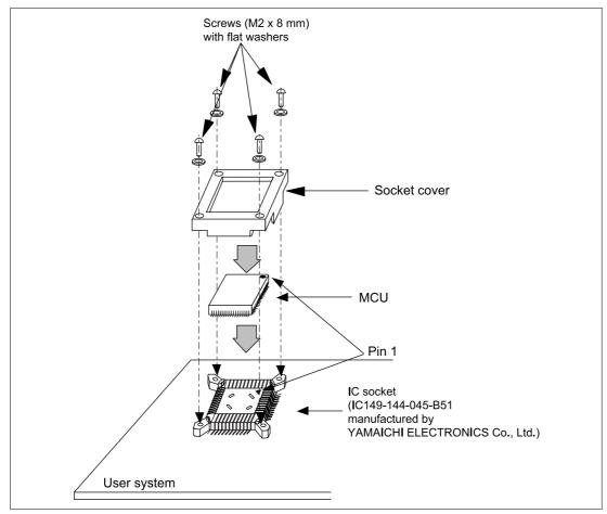
Figure 8 Installing MCU to User System
